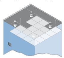
Sound masking technology consists of a series of loudspeakers installed in a grid-like pattern in the ceiling, as well as a method of controlling their zoning and output. The loudspeakers distribute an engineered sound, maintaining the facility's ambient level at an appropriate and consistent volume. Though the sound is similar to softly blowing air, it's specifically designed to mask the frequencies in speech. It also covers up other noises or reduces their disruptive impact on occupants.
